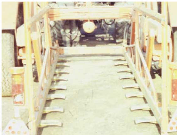
Fig. 14. Pyro-s trailer: grips securing box pallets
