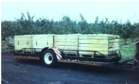
Fig. 10. Self-unloading trailer with 4 pallets (source: Rabcewicz, 2001)
