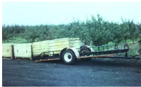
Fig. 11. Sliding of pallets from self-unloading trailer (source: Rabcewicz, 2001)
