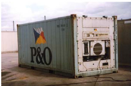
Fig. 64. Refrigerated container with fresh air supply and controlled atmosphere
