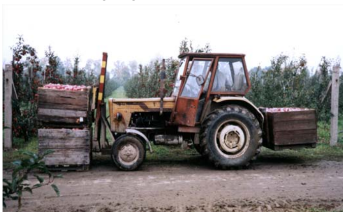
Fig. 9. Tractor with forklifts during work in orchard (source: Rabcewicz, 2001)
