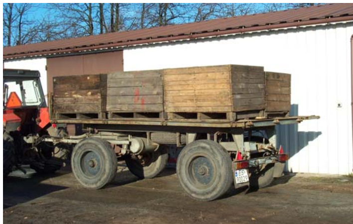
Fig. 16. Two-axle box-type trailers, D44B, with a loading capacity of 3.0 t
