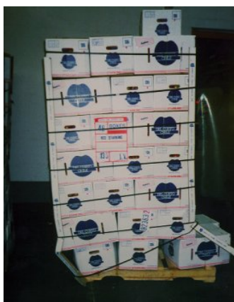
Fig. 66. Packages with apples of this cargo was not correct secured against impact at travel in storage facility (source: http://www.tis-gdv.de )
