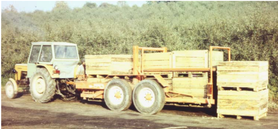
Fig. 15. Pyro-s trailer: loading of box pallets
