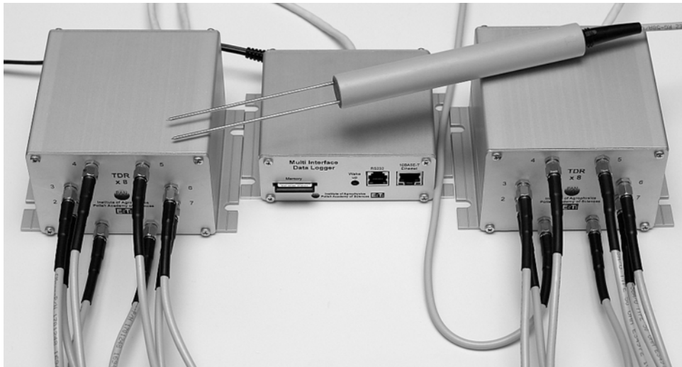
Fig. 9. Multi Interface Data Logger (in the middle between TDR soil water content, salinity and temperature meters) in the configuration for the measurement of 16 TDR FP/mts probes
