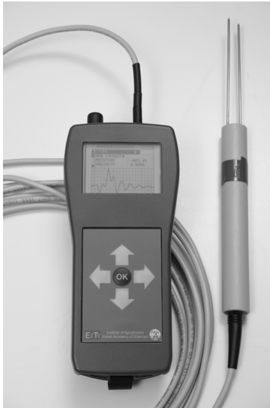
Fig. 12. Prototype of a handheld soil water content, salinity and temperature meter constructed with the application of modern components
