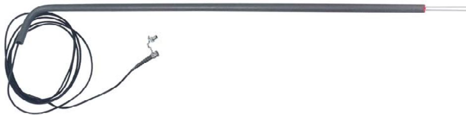
Fig. 13. FP/m, FP/mts - Field Probe for water content, temperature and salinity of soil developed in the IAPAS, Lublin
